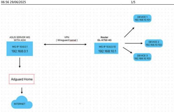
Our solution bases on the GL router, including the VPN Server and Client. Only for reference.
