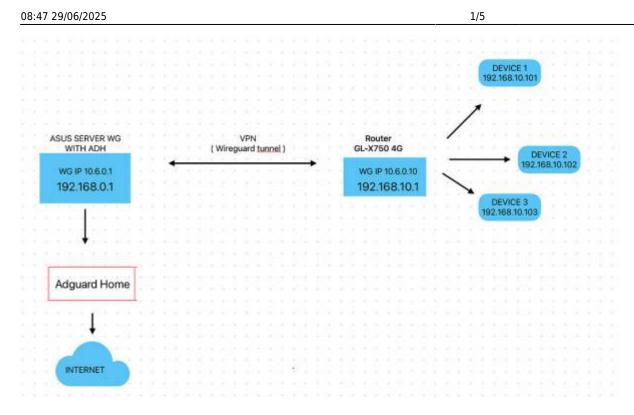
Our solution bases on the GL router, including the VPN Server and Client. Only for reference.
